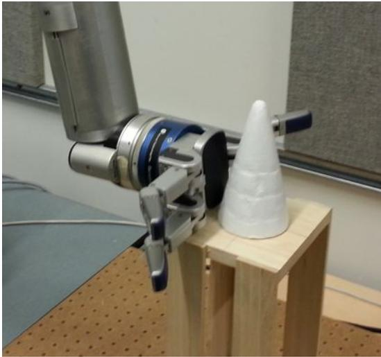
Thus, each grasp is a combination of two factors: the position of the hand and the position of the fingers. The position of the hand, referred to as the "target position", can be either from the side (side-on) or from above (top-down). The position of fingers 1 and 2 can be at  $0^\circ$  (prism),  $30^\circ$  (tripod), or  $180^\circ$  (wrap). When the user chooses one of the above grasps, the robot follows a fixed sequence of states:
